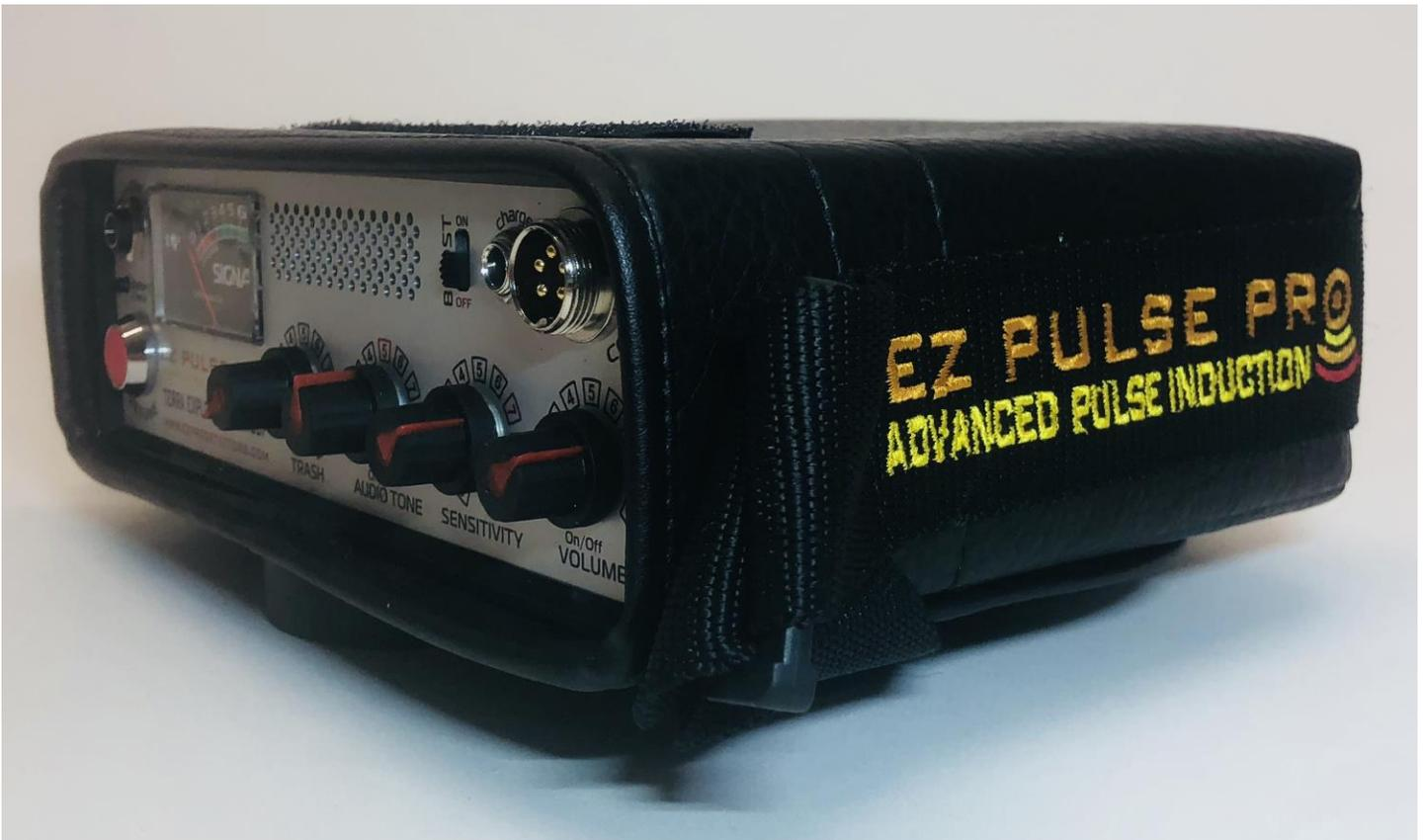
**1.1 Electronics Unit** has a built-in 12.0V/2600 mAh NiMH battery, providing up to 8 hours continuous use per battery charge. The electronics unit is housed in a protective leather case with an around-the-neck carrying strap. Never remove the electronics unit from the leather case as the unit can be damaged and the warranty will be void.
