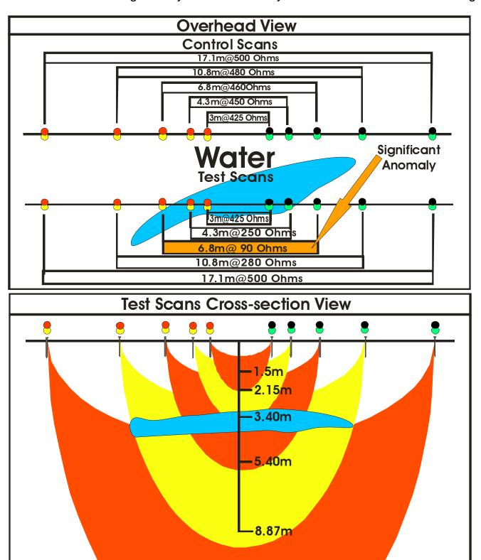
**3.** How to find metallic mineral veins or large metal caches: The illustration below shows overhead and cross-section views of a two-probe resistivity array in a hypothetical search for a metallic mineral vein. The methodology is exactly the same as explained in the water example whereby resistivity at some depth will exhibit a **very significant decrease** in resistivity numbers as metallic mineral veins are always more electrically conductive than the surrounding normal soil.
